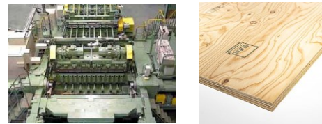
Rotary lathe peeling small diameter soft wood log
